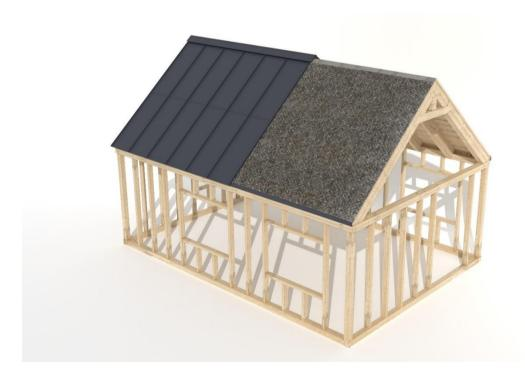
Once Ventia Metal Underlay has been installed and secured, the installation of the metal cladding can proceed. Ventilation is required from the eaves to the ridge for all situations.
