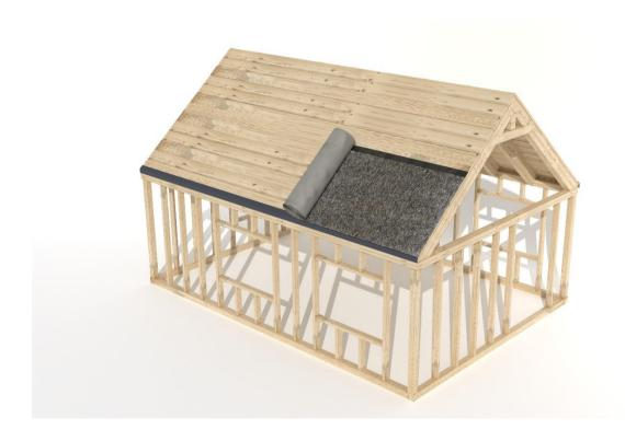
Ventia Metal Underlay should be placed directly on clean and dry plywood sarking or OSB panels.
