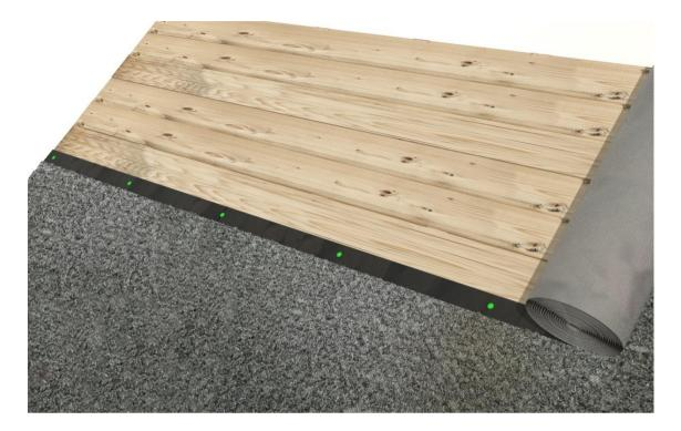
The underlay is fastened to the boarding with roofing staples. Ventia metal Underlay should be laid with a minimum overlap of 150mm.
