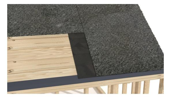
Any vertical joints of two membranes must have a minimum overlap of 200mm. Remove accordingly the drainage layer along the entire width from one of the membranes allowing the section to meet the required minimum overlap of 200mm and to be glued together.
